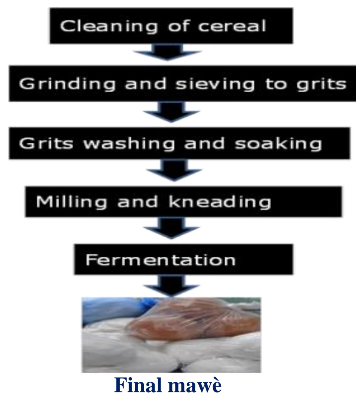
Fig. 1. Flow diagram of mawè production. The grits is not washed in home mawè processing. In come mawè processing, the cleaned maize is directly soaked in boiled water without grinding.
